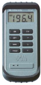
An economically priced thermometer with a Type K sensor which extends the upper measurement range to 1300°C. It incorporates a useful maximum temperature memory function and comes complete with a slipon rubber boot.
