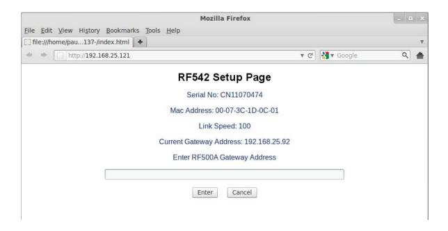
6. In the box provided type in the IP address of the RF500A Gateway that will store the data for this transmitter. The IP address for the RF500A Gateway should be provided by your IT Department.
