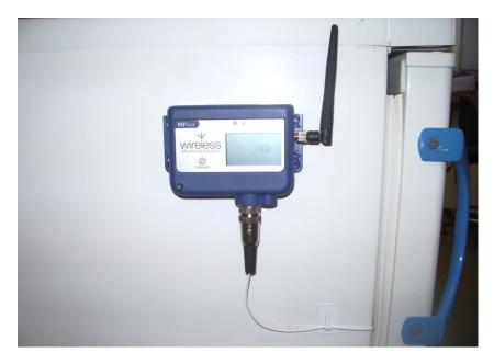
Note: Wherever possible use a dedicated port to run the external probe into the equipment (ie Incubator, Freezer, Fridge). If you wish to mount the transmitters on the inside of any equipment please make sure that this is the way that the system was surveyed. It is very important that the position of the transmitters is exactly as it was during the survey to be sure that the system will work.
